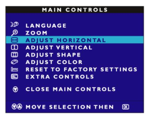
3) Press the **log** button. The ADJUST HORIZONTAL window appears. POSITION should be highlighted.
